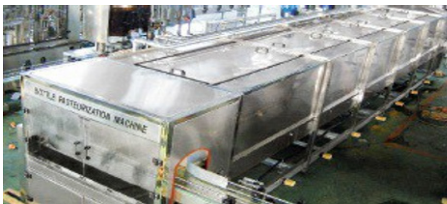
Figure 1: continuous pasteurizer in a tunnel through which the already packaged food is treated.
